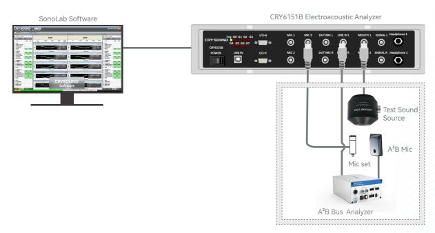
During testing, SonoLab software controls the CRY6151B Electroacoustic Analyzer to generate specific audio signals. These signals are converted into sound via a test source, while a reference microphone set ensures measurement accuracy. The DUT Mic on the A<sup>2</sup>B bus captures the sound, communicates with the A<sup>2</sup>B Bus Analyzer, which decodes the signal and outputs analog audio to the analyzer for further analysis.
