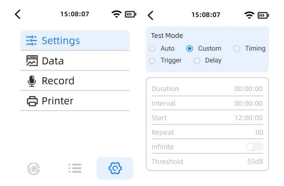
When users switch to the "Settings" interface, they can configure the test mode, view data playback, set recording options, and choose printing methods.
