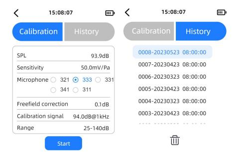
Users can click "Calibration" to enter the "Calibration" app. The "Calibration" interface displays the current sound pressure level and the microphone sensitivity. Users can set the microphone model, and the corresponding free-field correction value will change accordingly, with CRY2834 defaulting to the CRY331 sensor and CRY2833 defaulting to the CRY333 sensor.
