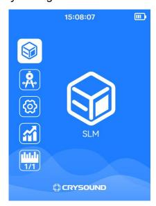
2) Press the power button for 3 to 5 seconds until the startup animation appears on the screen. The screen will then display the measurement main interface.
