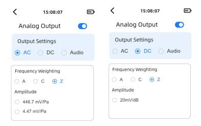
When "Analog Output" is selected by the cursor, pressing the confirm button enters the Analog Output interface.
