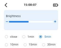
In the "Display Settings", users can adjust the screen brightness using the left and right buttons, and set the screen timeout below. The device defaults to 50% brightness and does not automatically turn off the screen.
