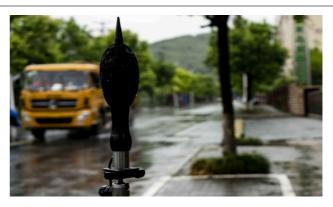
The CRY2833 and CRY2834 sound level meters, when used with the N41 protector (IP65), automatically record and transmit real-time data when noise exceeds set thresholds, creating an auditable trail of noise events.
