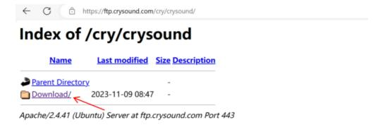
Click "Download", it will display the materials available. Click "Firmware", it will show the firmware for different models. Click "CRY2624", download the firmware inside. Save the downloaded firmware in the microSD card.
