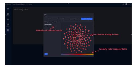
After the self-test is completed, each channel displays its sound intensity value in dBSpl, and the channel color corresponds to the color map bar below. The color bar is 0–120dB from left to right.
