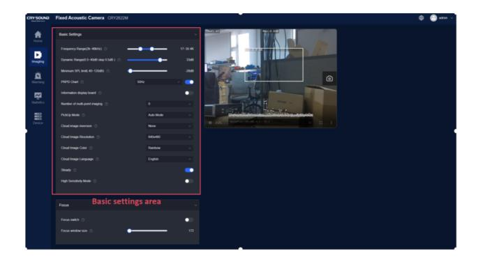
Frequency Range: Set the frequency range of the sound in the environment picked up by the microphone array. The range is 2k-48kHz, and the maximum difference between the upper and lower frequency limits is 2kHz.
