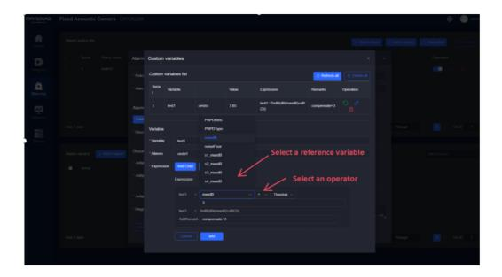
3.2. Select the type of value to be calculated, which is divided into two types: real-time value and threshold, where the real-time value is the reference variable in 3.1 above, and the threshold value is the manually entered value, as shown in the following figure:
