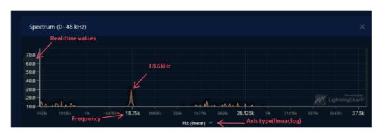
FFT: The frequency-amplitude curve calculated from short-time Fourier transform of the raw audio data;
