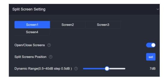
Choose a split screen, as shown in the figure, the selected split screen is Split Screen 1 **Enable/disable Split Screen:** Toggle the Split Screen on/off.
