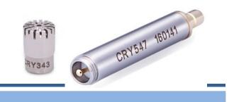
CRY343 measurement microphone is a pre-polarized 1/4 inch free field condenser microphone. It mainly used for high-level and high-frequency measurements since the sensitivity is low. It can measure high sound pressure levels to 164dB. The titanium diaphragm can achieve high stability and accuracy in harsh environment.
