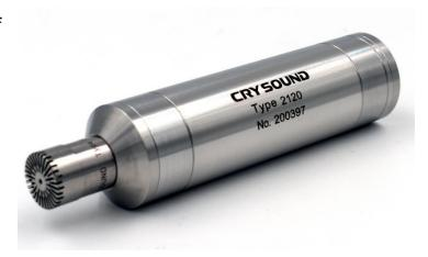
CRY2120 noise sensor integrates measurement microphone, preamplifier, high-precision ADC, high-speed DSP processor and excellent hardware design which provides 110dB dynamic range and can measure lower to 25dBA environment noise. The sensor has a compact structure with small appearance, the stainless-steel shell gives a perfect corrosion resistance.
