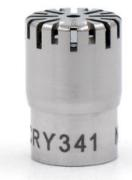
Its sensitivity is  $4mV(-48dB) \pm 3dB$  @250Hz and the frequency response is  $4Hz - 40kHz \pm 2dB$ .
