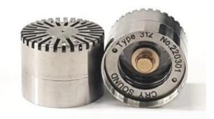
The CRY312 microphone is a type I pre-polarized 1-inch pressure field measurement microphone that converts acoustic signals into electrical signals. Using titanium film and special materials, and special stability treatment, has the advantages of wide frequency range, good frequency characteristics, wide dynamic range, good dynamic characteristics, good temperature and long time stability, especially suitable for high frequency and high noise pressure level measurement.
