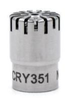
Its sensitivity is 15.8mV(-36dB)  $\pm 2$ dB @250Hz and the frequency response is 4Hz - 40kHz  $\pm 2$ dB.
